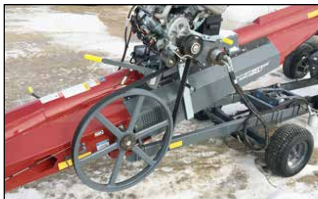
Fig 21 - Larger drive-to-belt pulley, shown with guard removed
